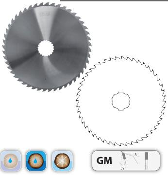
Special saw blades with the central bore type Spline & Can-Drive with flat (GM) or alternate top bevel (GS) teeth. Saw blades with hard, properly chosen carbide or stellite tips designed for cutting fresh (wet and frozen) wood. Ripping saw blades are equipped with special design of chip breaker, to guarantee optimal work efficiency of the tool.
