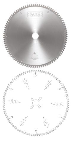
Saw blades with medium and high teeth number and triple-chip + flat teeth (GA), type **PI-530** with special carbide tips, designed for precise cutting of profiles and thin light alloy and plastics sheets on manual feed machines and automatic lines.
