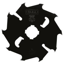
Upgraded multi-rip saw blades, type **PI-515 EVO** with flat (GM) or alternate top bevel (GS) teeth and carbide tips, designed for longitudinal cutting of wet, soft wood with low feed (up to 10 m/min) on a multi-saw blade machine. Special body coating technology prevents the resin from sticking to the blade and reduces the blade-wood friction.
