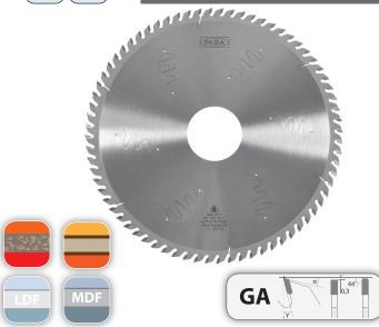
Panel sizing saw blades with medium teeth number and group triple-chip + flat teeth (GA), type **PI-521VT**, with very hard carbide tips (T), designed for cutting chipboard, laminated board, LDF and MDF in stack.
